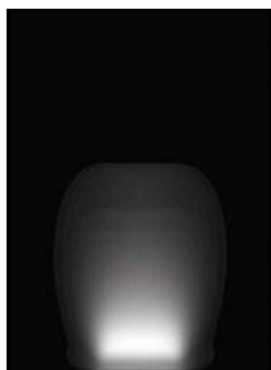
Light distribution Narrow spot 32°
